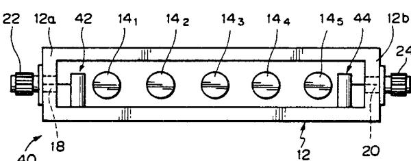
**Hermetically Sealed Oscillator with Dielectric Resonator Tuned through Dielectric Window by Adjusting Screw**
